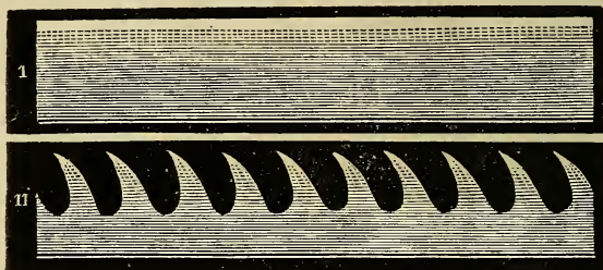
FIG. 184.—Appearance of the flame in the mirror of König's apparatus. 1, organ pipe not sounding; 2, organ pipe sounding,—the teeth representing individual vibrations of the air in the pipe.
